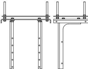
TA - TORQUE-ARM II Shaft Mount Reducer
