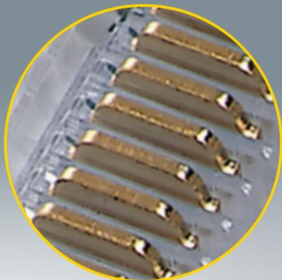
Thin, pitted, uneven plated surface leads to premature erosion of contact and causes connector failure.
